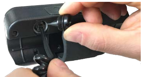
Figure 14 - Unplugging the connector
