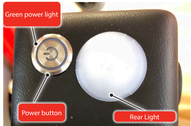
Front and Rear lighting system
